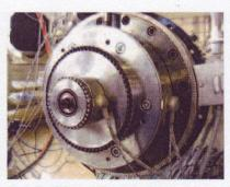
Fig. 3. Two-channel die with an integrated flexring sleeve for fine adjustment of the layer thickness of the outer layer (rear adjusting screws) and the overall thickness (adjusting screws at the die mouth)
