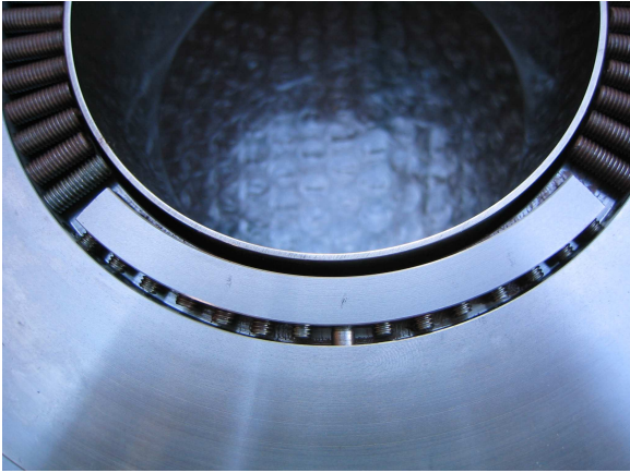
Fig. 3 Adjustment jaw with integrated grub screws for fine setting of the active setting jaw contour
