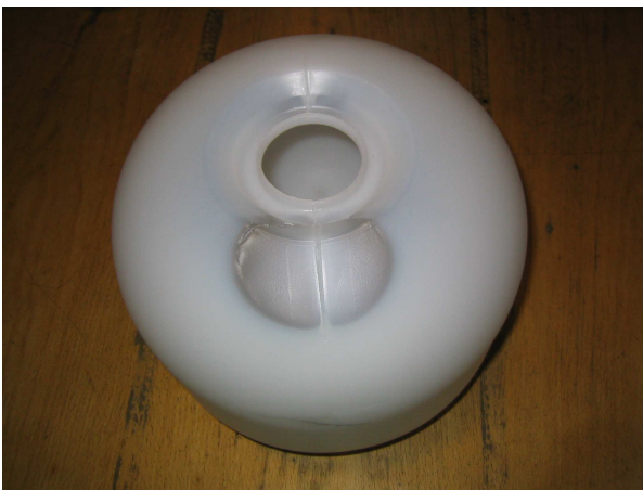
Fig. 4 Blow moulded bottle with extreme thin area which has been generated for the purposes of demonstration by short term local closure of the flow channel gap on the die by means of the setting jaw
