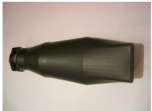
Fig. 6 Special designed bottle with varying cross-sectional geometries manufactured with the test die (photo IKV)
