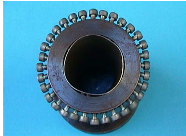
Fig. 1 Cross sectional drawing of a flex ring die (right side) and Photo of an outer ring with an integrated flex ring sleeve (left side)
