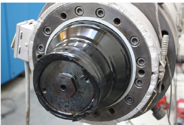
Figure 1. Tilting joint that has been retrofitted into the parting plane between the head and the die
