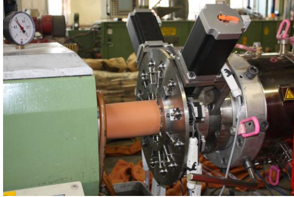
Fig. 4 Flex Ring die combined with tilting technique which enables to establish a closed-loop control to minimize as well eccentric, as also asymmetric variations in the thickness of extruded pipes
