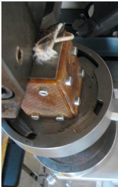
**Fig. 3. Bayonet lock coupling of a capillary die with tilting technique**
