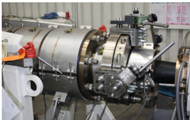
**Fig. 4. Pipe head with a retrofitted tilting die. For tilting it has only two adjusting units sitting at a 90° angle to one another. Though operated via large adjusting screws, the screws' adjustment travel is very finely tuned, thanks to downstream mechanical gear reduction**
