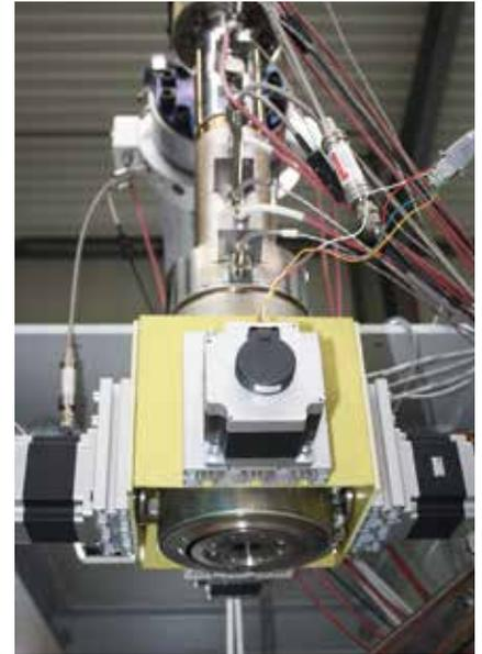
**Fig. 8.** Compact autonomous GWDS die head with integrated tilting joint: Both the translational stroke movement and the tilting movement of the die were realized using identical stepper motors (© H. Gross)
