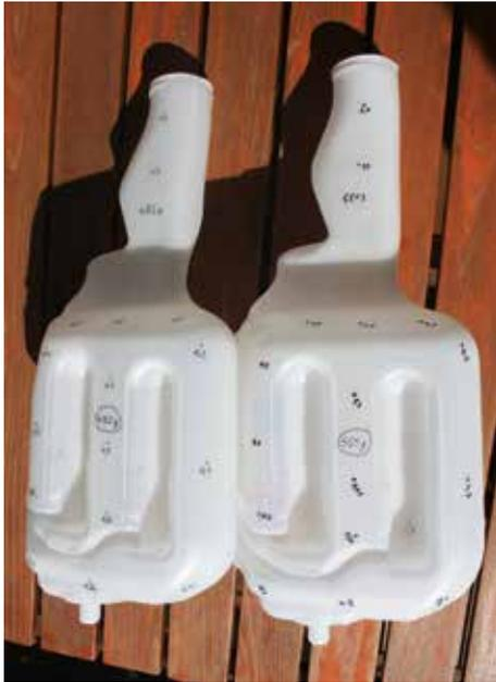
**Fig. 2.** Fabricated windshield washer reservoir using GWDS wall thickness control technology (left) with optimized wall thickness distribution, it weighs 482g compared to 560g in conventional production (right)
