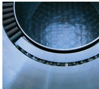
Fig. 3. Adjustment jaw with integrated grub screws for fine setting of the active setting jaw contour
