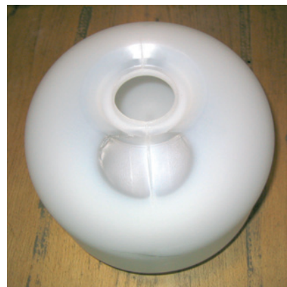
Fig. 4. Blow-moulded bottle with extreme thin area which has been generated for the purposes of demonstration by short-term local closure of the flow-channel gap on the die by means of the setting jaw
