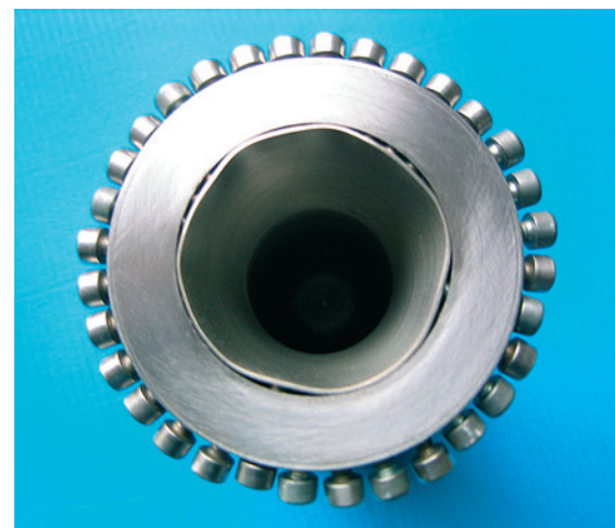
Fig. 1. Test die with 32 setting screws in which the flex-ring sleeve is subject to extreme purely linear elastic deformation for demonstration purposes
