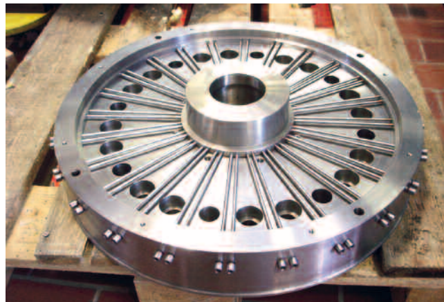
Fig. 4. Coextrusion sheet die made in one piece, with integrated, partially multiwalled flow-channel wall and radially disposed adjusting screws for fine adjustment of the local flow-channel gap in the region where the middle and inner layer flow together
