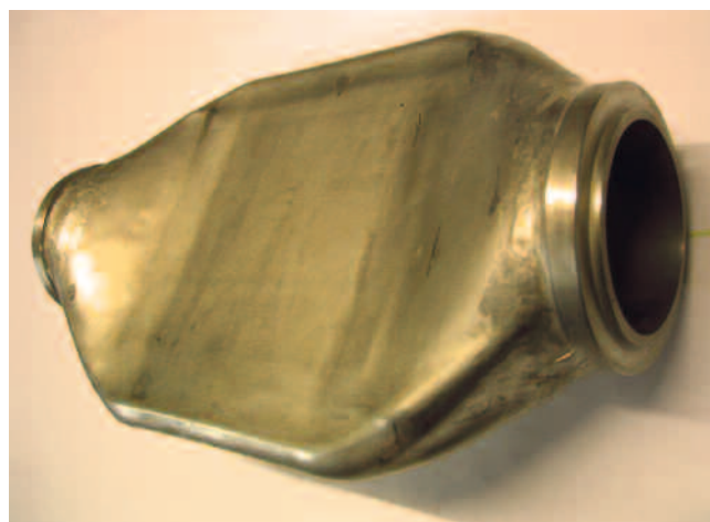
Fig. 7. Throttle body with the continuous transitions from the central flat flow-channel geometry to the respective circular inlet and outlet geometries
